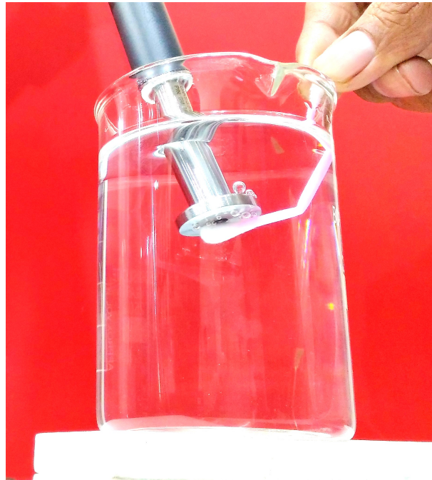
Figure 1.6: Removal of air bubbles from DAK probe immersed in liquid
